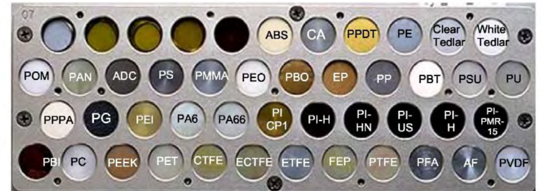
Figure 2.—Photograph of the MISSE 2 PEACE Polymers experiment prior to flight. The labels shown indicate the materials defined in Table I.
