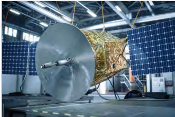
Engineering plastics with low outgassing, wide operating temperature ranges, and resistance to radiation and erosion from atomic oxygen are used for state-of-the-art satellites.
