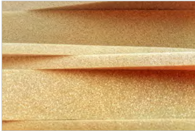
Aerospace-grade rigid polymer foams are seeing increased use for applications where light weight, thermal insulation, and acoustic insulation are required.
