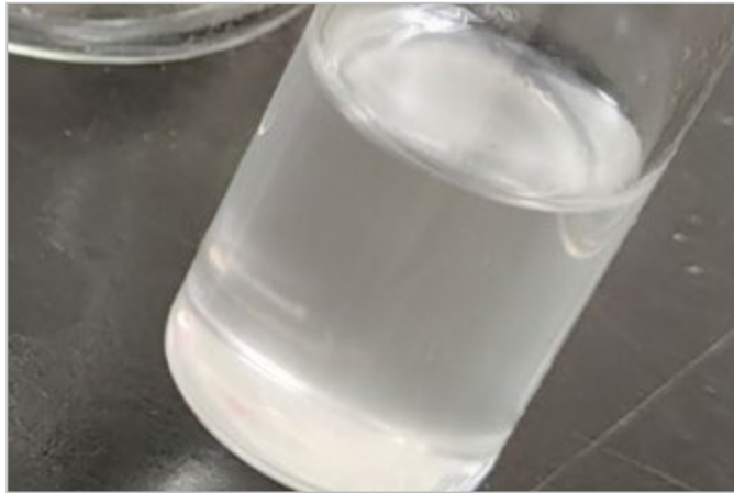
Figure 6: Solvent (xylene) Containing Dissolved HDPE After Heating for 5 Minutes at 104^\circ\text{C}
