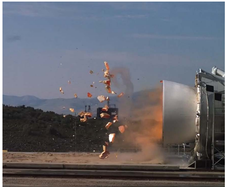
Image of GP's foam used as nozzle closure that protects a rocket's motor from environmental factors until ignition. Closure then breaks apart when motors are ignited.
