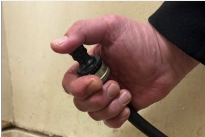
Relaxing thumb pressure on a garden hose releases water. This is analogous to the failure of a plastic seal due to stress relaxation.
