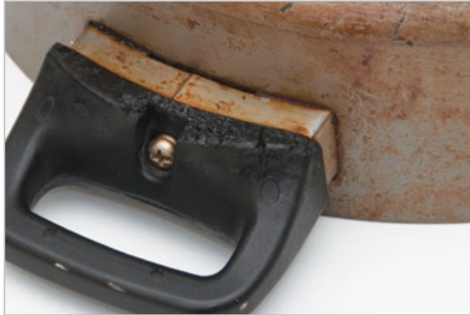
This phenolic pot handle became brittle and degraded after many years of use at elevated temperatures.
