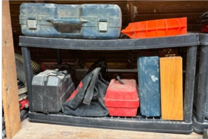
Plastic shelving that deformed over time due to flexural creep strain.
