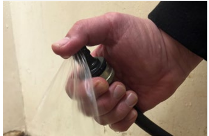
Relaxing thumb pressure on a garden hose releases water. This is analogous to the failure of a plastic seal due to stress relaxation.
