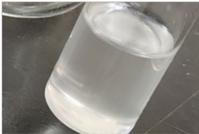
Solution of solvent (o-xylene) containing dissolved HDPE after heating for 5 minutes at 104°C.
