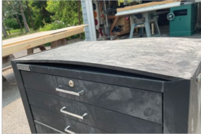
This HDPE tool chest top warped when placed outside on a warm day due to its high rate of thermal expansion.
