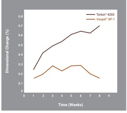
Figure 10. Dimensional Changes for Vespel® SP-1 and Unfilled Torlon® 4203 PAI Over a Period of 8 Weeks at 100 °F with 90% Relative Humidity
