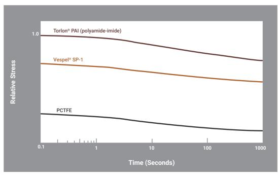
Figure 3. Stress Relaxation of Vespel® SP-1, Torlon® PAI, and PCTFE in Compression at 10% Engineering Strain at 299 K
