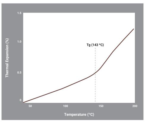
Figure 4. Thermal Expansion Curves for PEEK Both Above and Below the Material's Glass Transition Temperature
