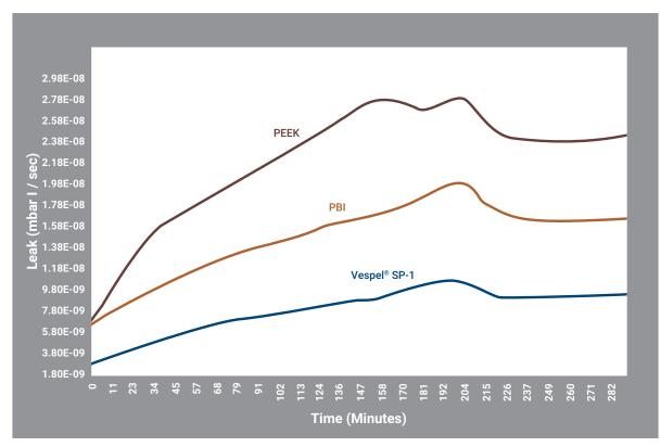
Figure 9. Vacuum Sealing Characteristics of Vespel® SP-1, PBI, and PEEK Measured via Helium Permeation at Room Temperature
