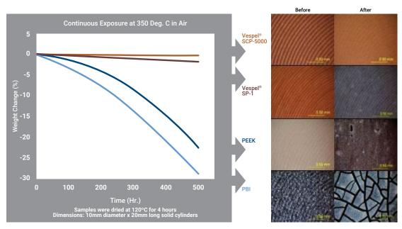
Figure 7. Resistance to Degradation at Elevated Temperatures for Vespel® SP-1, Vespel® SCP-5000, PEEK, and PBI
