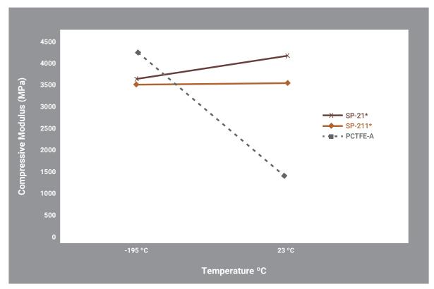
Figure 1. Compressive Moduli of PCTFE, Vespel® SP-21, and Vespel® SP-211 at Various Temperatures
