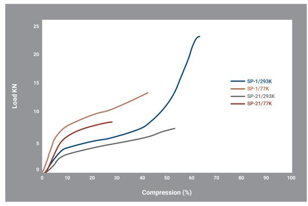
Figure 8. Ductile Compressive Strain of Vespel® SP-1 and SP-21 at 77 and 293 Kelvin
