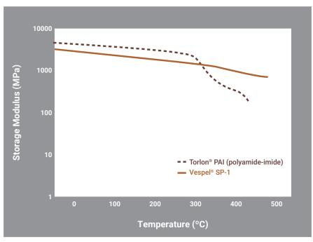
Figure 6. Storage Modulus of Vespel® SP-1 Compared with Torlon® PAI
