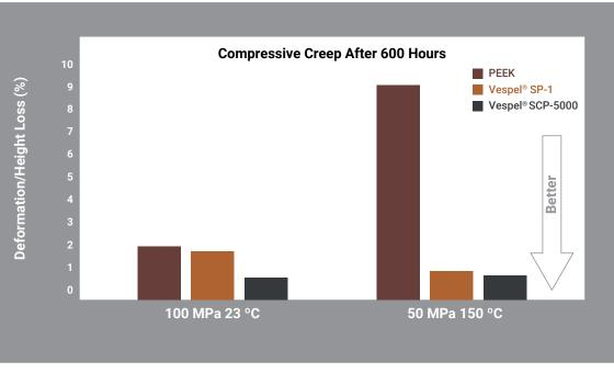
Figure 2. Creep Strain of Vespel® SP-1, Vespel® SCP-5000, and PEEK
