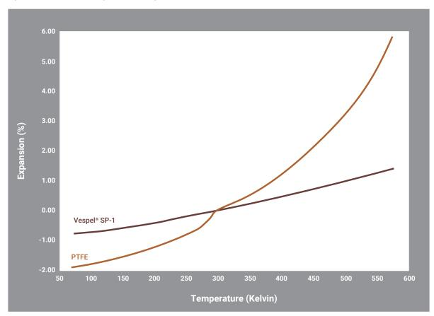
Figure 5. Linear Thermal Expansion of Vespel® SP-1 and PTFE from 73 K to 573 K
