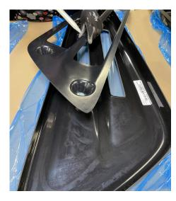
SCIGRIP 400LSE is a twocomponent (10:1), translucent, methyl methacrylate adhesive for bonding polyolefins with no surface preparation required. It bonds polypropylene, polyethylene and has the ability to cross-bond to metals like aluminium and stainless steel. Product is non sagging, and has short fixture times, making it an excellent choice for assembly and other fabrication or manufacturing uses.
