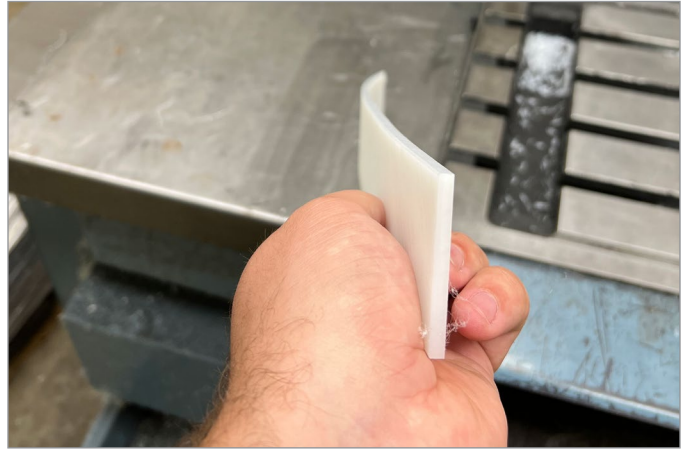
This UHMW-PE wear rail warped during machining due to residual stress in the sheet material.
