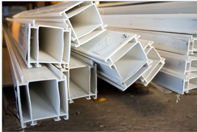
These PVC extrusions warped from creep strain due to improper storage.
