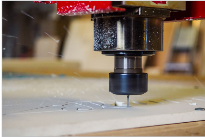
The mechanical action of cutting tools introduces frictional heat to plastic parts and also deforms the parts to some extent during machining operations.
