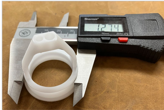
This injection molded acetal component exhibited post mold shrinkage, resulting in the part being outside of the specified dimensional tolerances.
