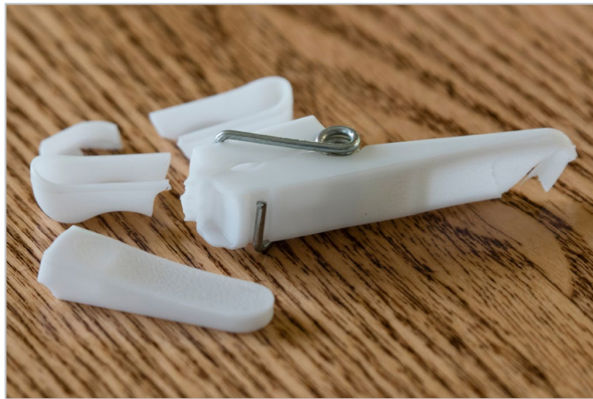
This laundry clothespin prematurely failed from flexural fatigue.
