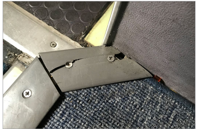
This plastic floor trim failed due to high hoop stresses from flat head screws.
