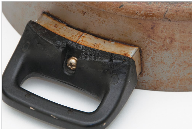
This phenolic cooking pot handle degraded and became brittle after long-term exposure to elevated temperatures during use.
