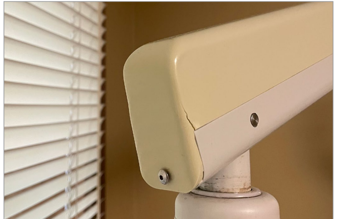
This ABS dentist office light housing failed from ESC. The sharp internal corner created a stress concentration. The cleaning chemical used in the office acted as a stress crack agent.
