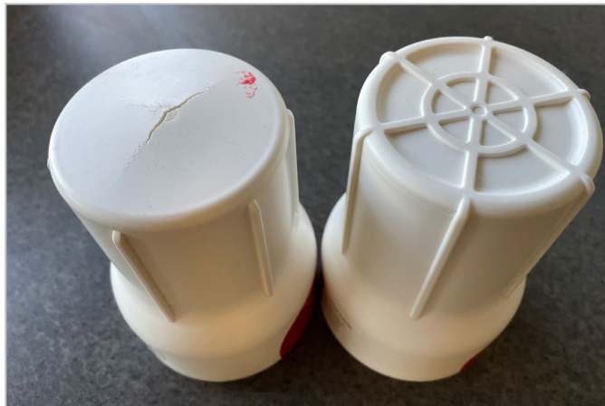
The filter housing on the left failed from creep rupture due to the internal pressure of the process fluid. The design of the housing on the right was modified to include reinforcing ribs for improved creep resistance.
