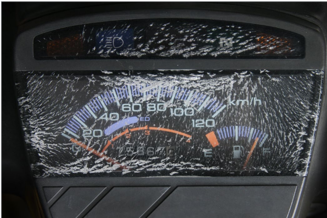
This acrylic speedometer lens failed from environmental stress cracking.
