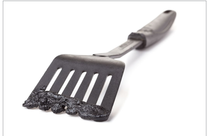
This plastic spatula softened when it came into contact with a hot metal cooking surface.
