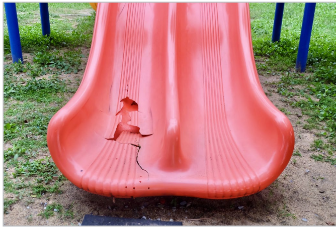
This polyethylene slide exhibited color shift from red to pink and it became brittle and cracked after years of exposure to sunlight.
