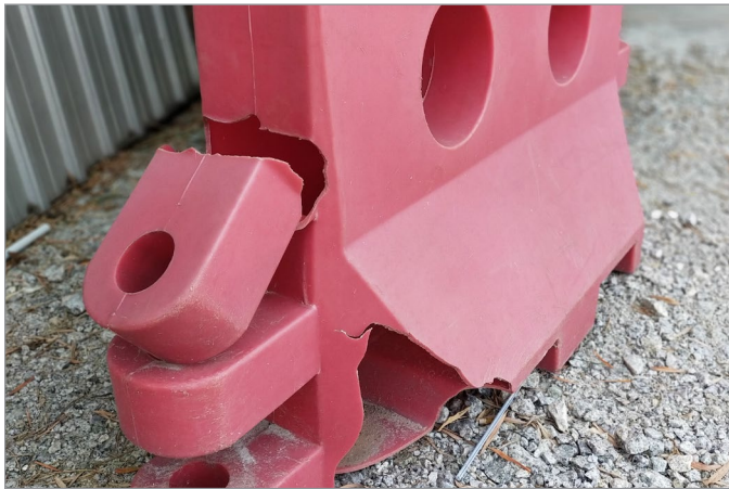
This construction barrier failed due to a stress concentration at a sharp 90 degree internal corner.
