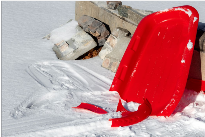
This polypropylene sled became brittle in cold winter temperatures and cracked during use.
