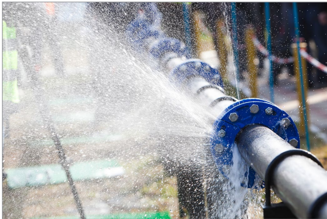
This metal piping was assembled using PTFE seals. These exhibited stress relaxation over time, which resulted in leak paths.
