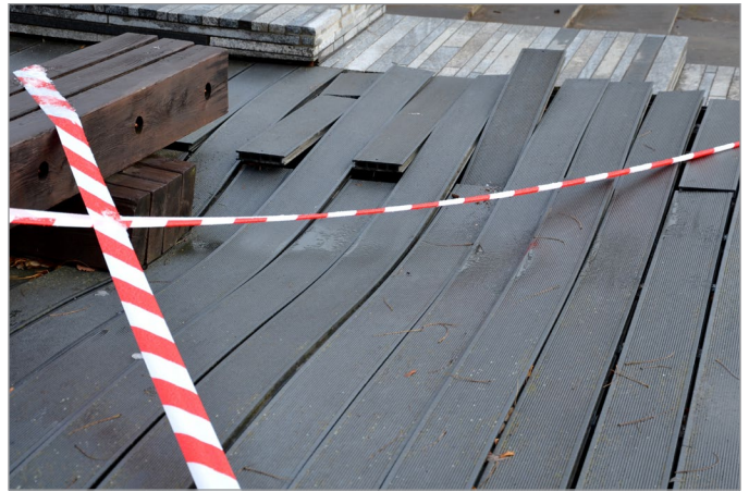
This HDPE decking was installed with insufficient support underneath, which resulted in the deck failing due to flexural creep strain.
