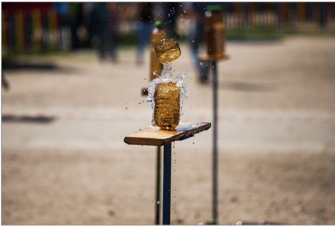
This PET bottle, which is tough and ductile in normal use, exhibited brittle fracture when exposed to the high strain rate impact of a bullet fired from a rifle.
