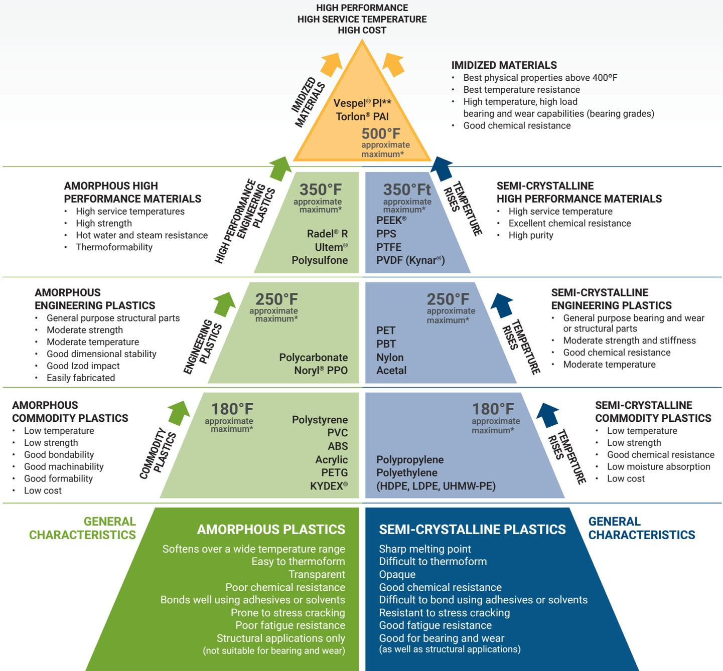
\*Materials should be considered for applications up to approximate maximum temperature. Selecting a plastic material for use in a high temperature environment requires careful review of material properties data. This chart is for comparison purposes only.
