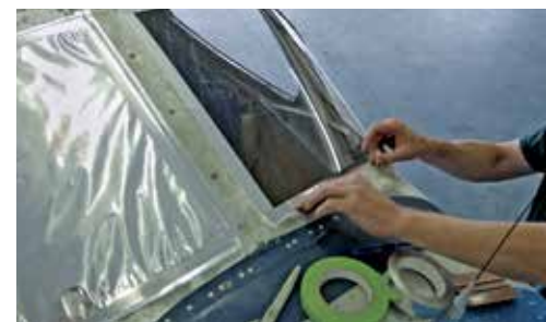
Plane paint masking
