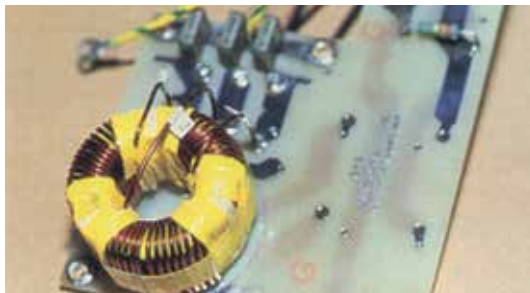
Coil outer wrap taping
