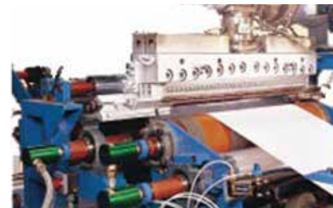
Orange overcoat masking tape on chill roll
