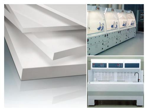
SIMONA® Polypropylene FRP-3 provides superior impact strength, rigidity and uniform white color in an FM 4910 listed sheet for semiconductor equipment. Among FR polypropylenes, it has an unmatched 12.0 ft-lb notched Izod impact, and 400,000 psi flexural modulus.
