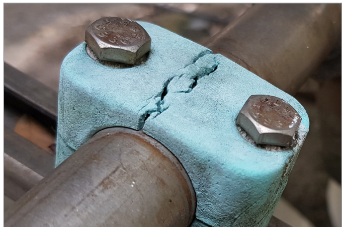
Creep rupture occurs in regions of high strain.
