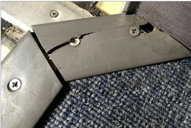
Threads and mechanical fasteners create high levels of stress and crack-initiation points in plastic parts.
