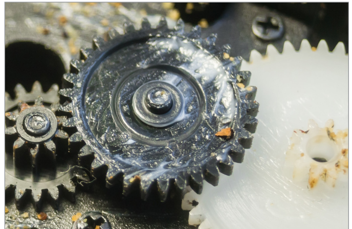
Self-lubricating gears and other mechanical components are often manufactured from semi-crystalline thermoplastics which are resistant to stress-cracking in industrial environments.
