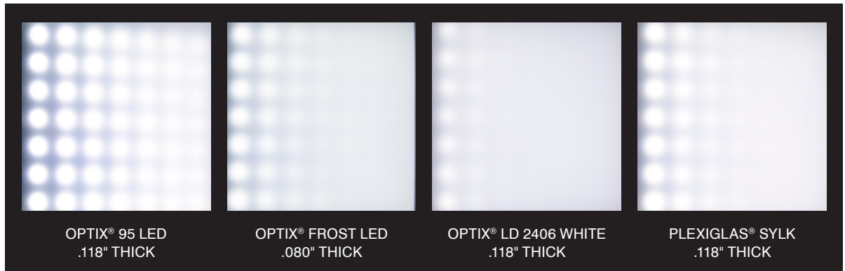
Figure 18. Acrylic diffuser materials backlit by LEDs set at depths from 0.50" to 1.75" from the surface of the light box.
