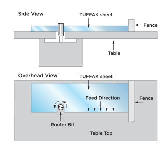
Important: Feed the sheet against the router bit rotation and use a fence for sizing when making straight cuts.
