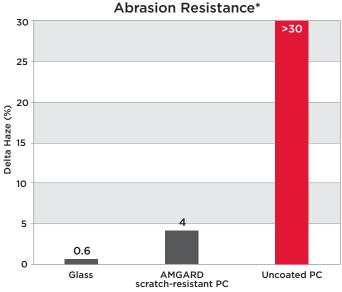
\*Taber Abrasion per ASTM D 1044, 100 cycles using CS-10F wheels at 500 g load
