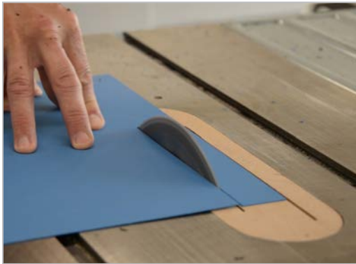
KYDEX® sheet is easy to cut using standard woodworking tools such as table saws and routers.
