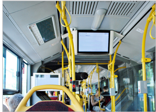
Pressure forming is an outstanding process for manufacturing parts, such as these ceiling panels, that require sharp definition.
