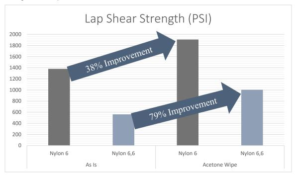
There are many different grades of nylon and as shown here, optimal results were created with Plexus MA8110 and Plexus MA8120. Also observed in this study is that Nylon 6 is easier to bond than Nylon 6,6. As a result, it is recommended that to ensure the ultimate bonding success, one should always thoroughly test and screen the particular grade of nylon being considered to bond, prior to final application.
