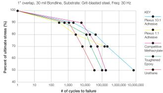
Not only does the adhesive joint provide a stronger bond than the rivet, but when tested in fatigue, Plexus adhesives outperform the riveted joint by over 98%.
