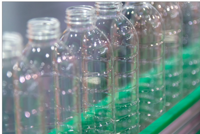
These green ultrahigh molecular weight polyethylene conveyor guides have low friction and long wear life against PET bottles. The soft surface of the polyethylene allows the machine to convey the bottles without scratching them.
