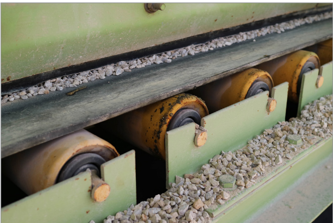
The plastic roller covers in this stone chip conveyor need to have outstanding abrasive wear characteristics due to gritty contamination from the stone.
