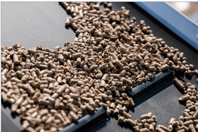
The plastic flights on this wood pellet conveyor need to have good abrasion resistance for long service life in extremely abrasive conditions.
