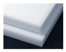
LDPE (low density polyethylene) is a soft, flexible, lightweight plastic material. It is often used for orthotics and prosthetics. LDPE has good chemical and impact resistance and is easy to fabricate and form.
