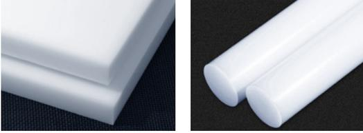
LDPE (low density polyethylene) is a soft, flexible, lightweight plastic material. It is often used for orthotics and prosthetics. LDPE has good chemical and impact resistance and is easy to fabricate and form.
