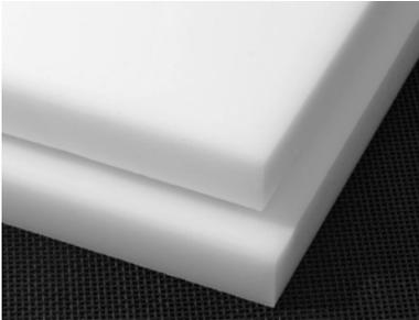
HDPE (high density polyethylene) is available in sheet for applications that require greater strength and stiffness than LDPE (low density polyethylene).
