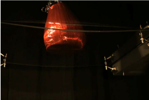
canopy test / tempered glass / 50 kg (110 lb)
