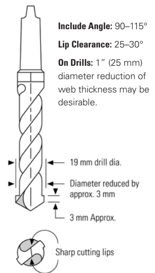
Figure 2: Modified Drill For Vespel® Shapes
