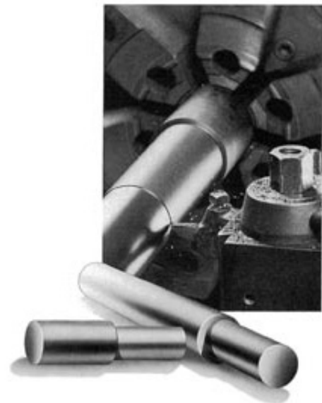
Turning cylindrical stock in a lathe
