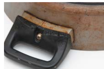
This plastic pot handle degraded and became brittle after many years of use at elevated temperatures.
