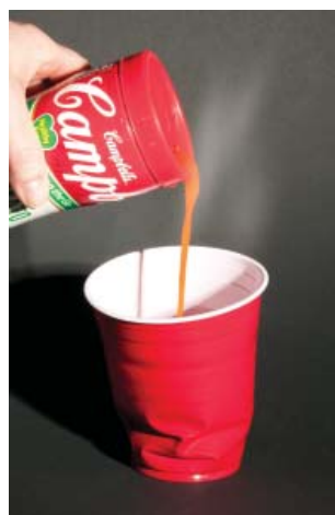
This plastic cup lost modulus (stiffness) and softened when it was filled with hot soup.
